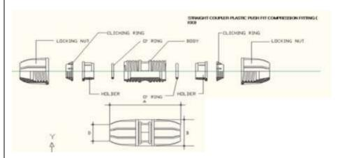
Standards : PP Push Fit Fittings in accordance to BS 5114, AS 4020 : HDPE PIPE PE 80 AND PE 100 ISO 4427 PIPE SUITABILITY WORKING PRESSURE: PN16 MATERIAL COMPONENT LIST : POLYPROPYLENE **BODY** RUBBER O'RING : NITRILE BUTADIENE RUBBER HOLDER : POLYPROPYLENE CLINCHING RING : ACETAL : POLYPROPYLENE LOCKING NUT Approx. wt 1/2" plastic coupler: 65 grams
