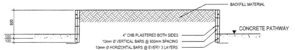
4 CONCRETE PLANT BOX DETAIL MIS-P/18 SCALE 1:37.5
