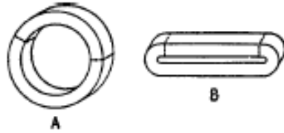
FIG. 5 Location of Transverse Tension Test Specimen in Ring Cut from Tubular Steel Products
