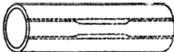
FIG. 4 Location from Which Longitudinal Tension Test Specimens Are To Be Cut from Large Diameter Tubing
